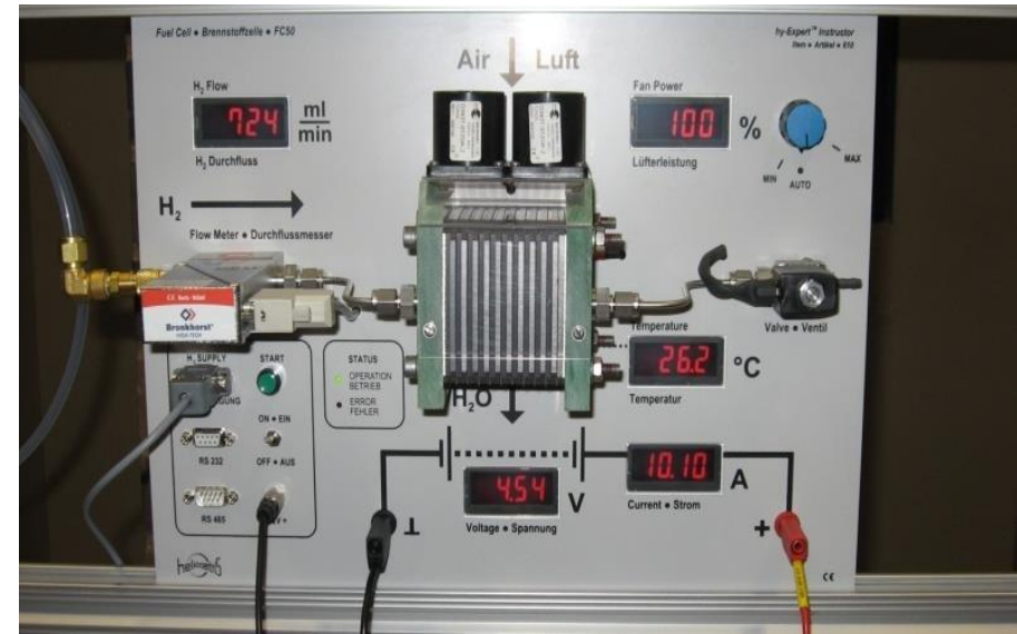
Hydrogen fuel cell
