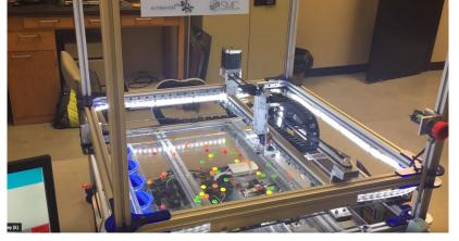
A) A two DOF belt driven robot must be designed to sort skittles by color
