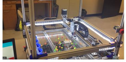
A) A two DOF belt driven robot must be designed to sort skittles by color
