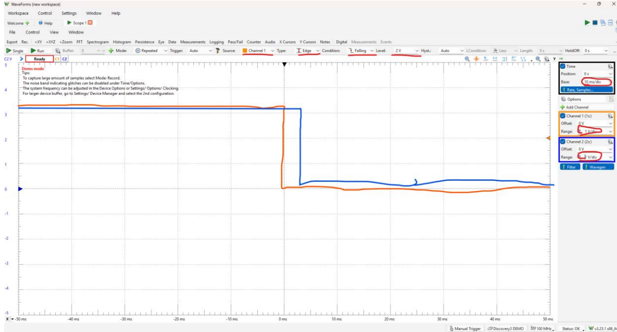
Figure 6 Setting up the oscilloscope to capture latency.
