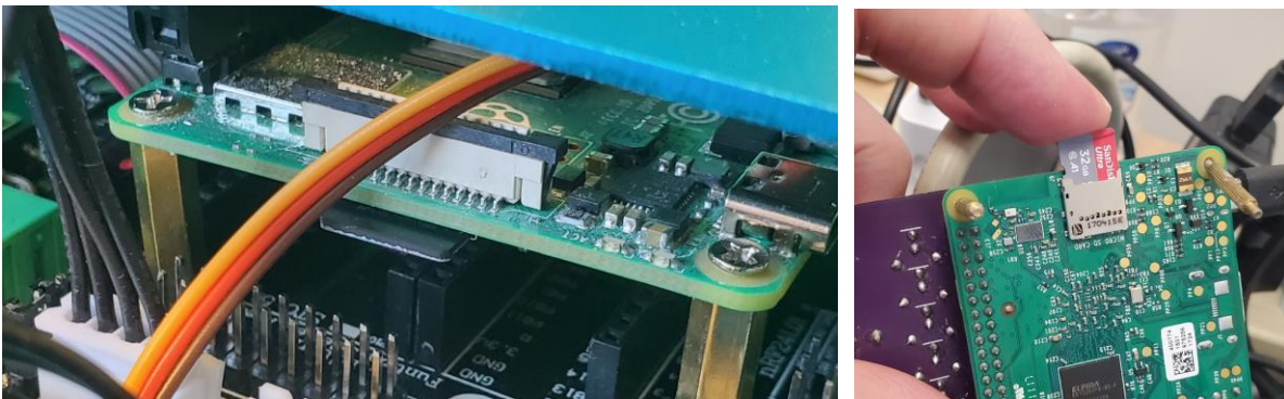
Figure 2 Inserting the uSD card into the Raspberry Pi. On the left we see the uSD card in the middle, right above the pins and under a display cable plug. On the right we see the card being inserted, looking toward the bottom side of the board.
