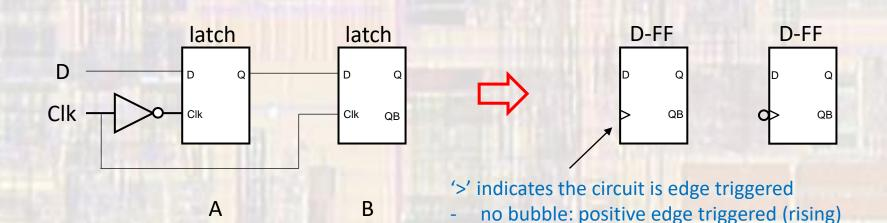
bubble: negative edge triggered (falling)
