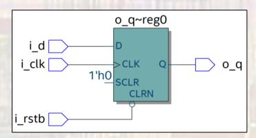
Most of our designs will use DFFs with an asynchronous reset
