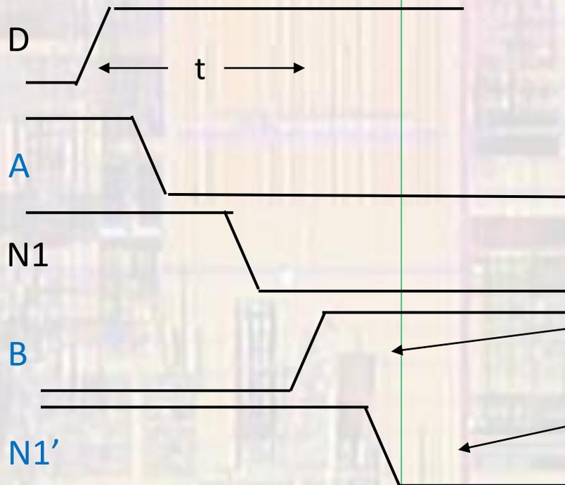
Proper operation requires the data to be stable for some amount of time before the clock rises  $\rightarrow$  SETUP TIME
