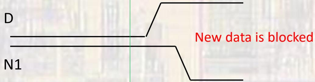
Proper operation requires the data to stay stable for some amount of time after the clock rises  $\rightarrow$  HOLD TIME
