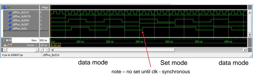
2 – Write behavioral VHDL code for a special new FlipFlop you have conceived of – this FlipFlop has a second data input called Toggle(T). When T is low, the DFF operates normally, when T is high, the DFF ignores the D input and synchronously toggles the output. Provide code and a simulation 50pts
