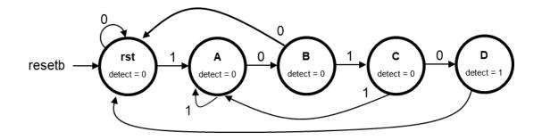
3 – Create output transition tables for the state diagram below using a) state names, b) binary encoding, c) one hot encoding and d) Johnson encoding. 20pts
