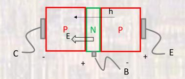
$$I_C = I_S \left[ e^{\left( \frac{V_{EB}}{nV_T} \right)} \right]$$
