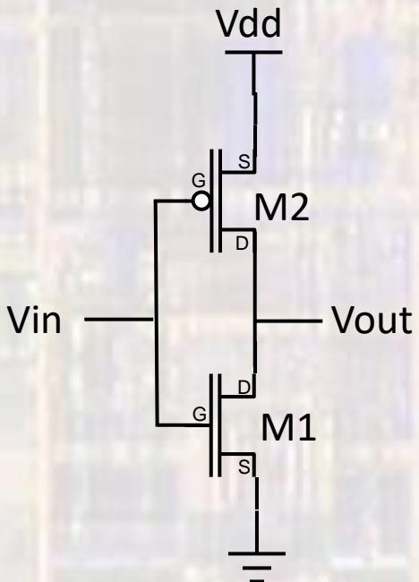
Assuming Vdd is big enough to keep M2 and M1 in saturation at the switching point
