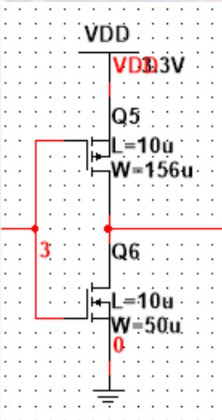
$$\begin{aligned}V_t &= 1V \\V_{tn} &= 1V \\V_{tp} &= -1V (1V) \\k'n &= 14\mu A/V^2 \\k'p &= 4.5\mu A/V^2\end{aligned}$$
