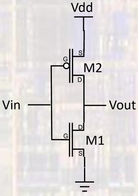
Desire a consistent switching point  $V_{in} = V_{out} = V_{dd}/2$
