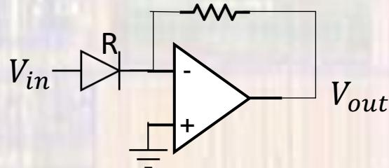
$$V_{out}/R = I_D = I_S e^{\frac{V_D}{nV_T}} = I_S e^{\frac{V_{in}}{nV_T}}$$
