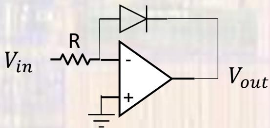
$$V_{in}/R = I_D = I_S e^{\frac{V_D}{nV_T}} = I_S e^{\frac{-V_{out}}{nV_T}}$$
