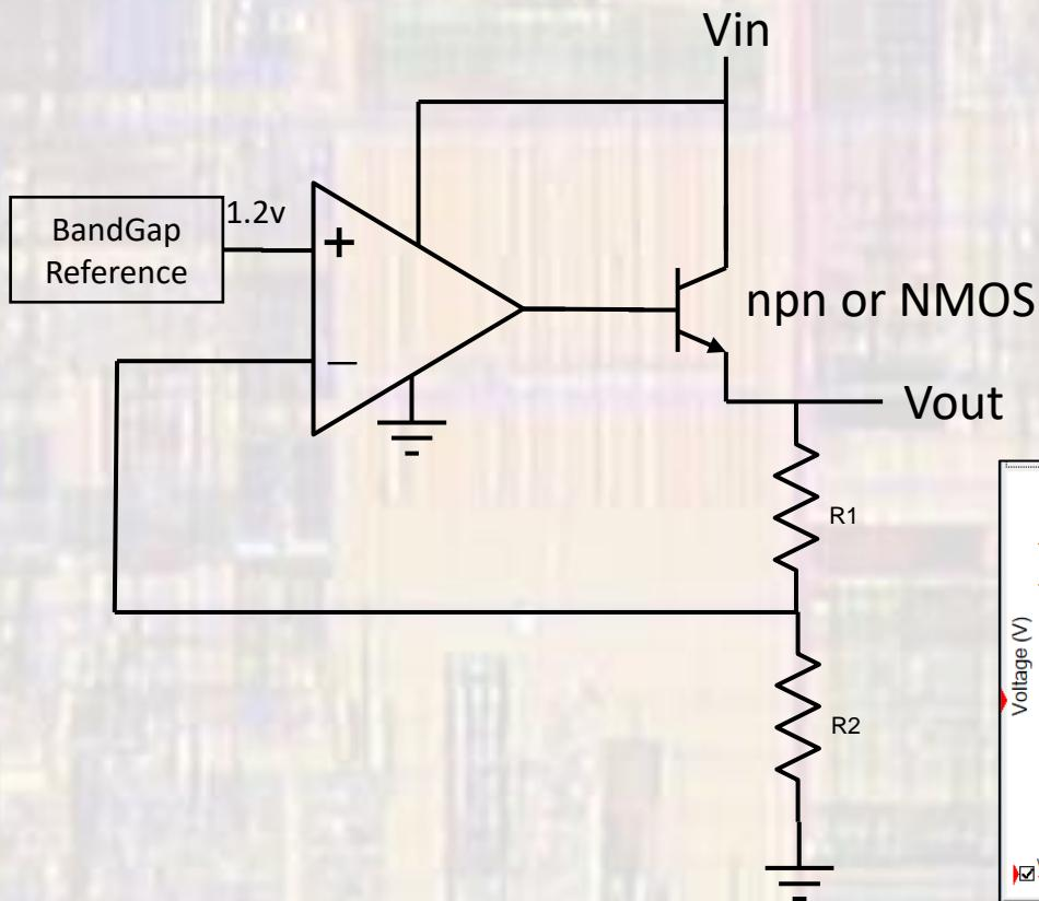
$$\frac{R_2}{R_1 + R_2} V_{out} = V_{bg}$$
