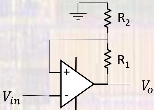
when  $V_o = vdd$ , then  $v_+ = vdd \frac{R_2}{R_1 + R_2}$
