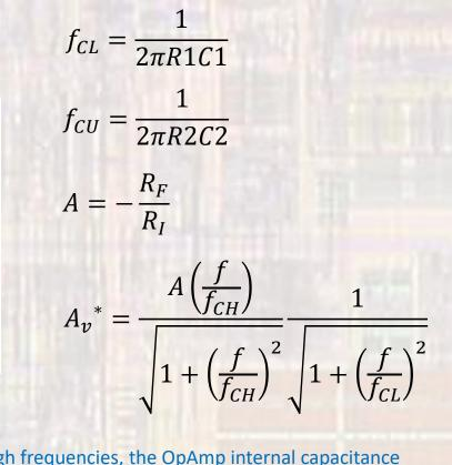
\* At high frequencies, the OpAmp internal capacitance limits the rolloff
