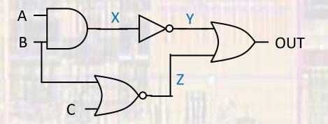
Out = Y + Z Out =  $(\overline{X})$  + (C + B) Out =  $(\overline{AB})$  +  $(\overline{C + B})$
