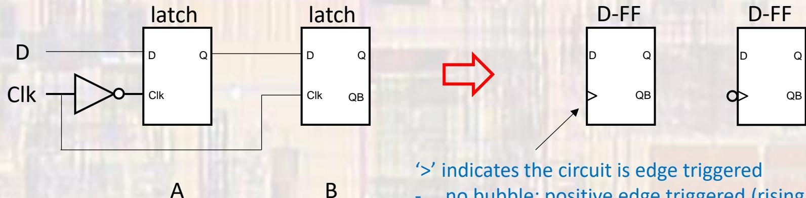
'>' indicates the circuit is edge triggered
