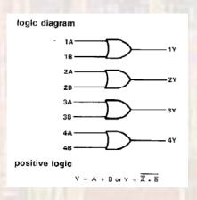
Note: The power for these parts is labeled  $V_{CC}$  – these are Bipolar ICs (Not CMOS ICs)
