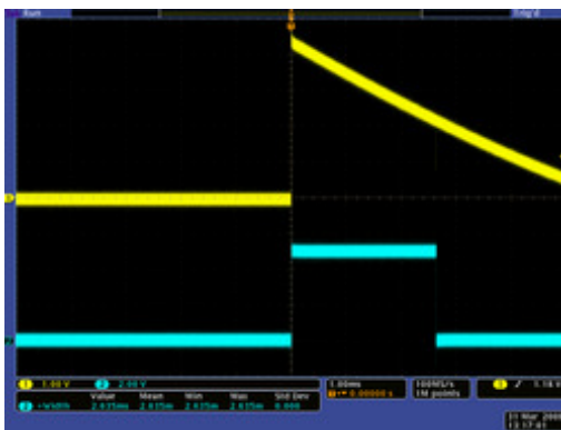
QTR-1RC output (yellow) when 1/8" above a black line and microcontroller timing of that output (blue).
