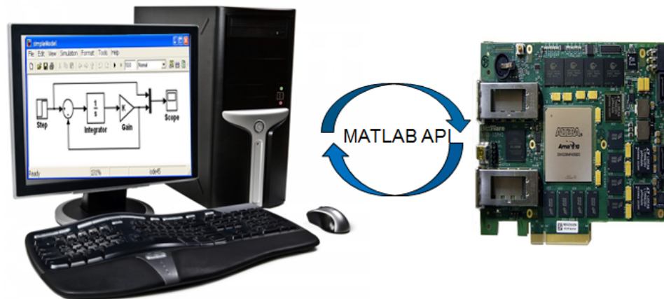
Figure 139. Hardware in the Loop Host-Target Setup
