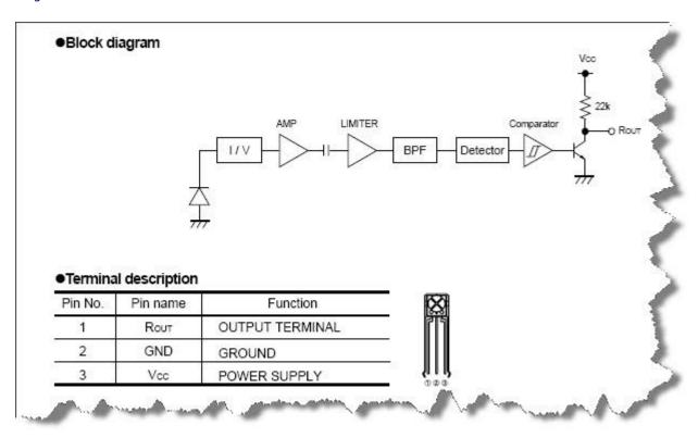
Output (Rout) is normally high as you can see from the block diagram, it has a pull-up resister that keep logic high when no signal present. When infra-red signal is detected, output is low.
