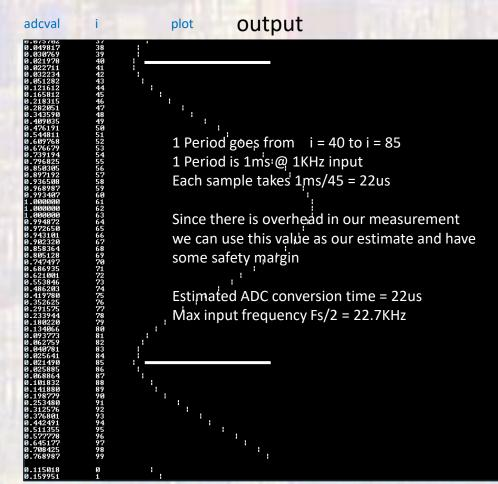
The actual ADC is capable of running much faster than this (5Msps)
