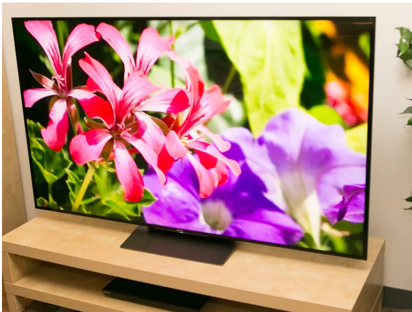
High-end LCDs like the Sony XBR-65X930D can get brighter than OLED TVs, which is especially important for HDR. Sarah Tew/CNET
