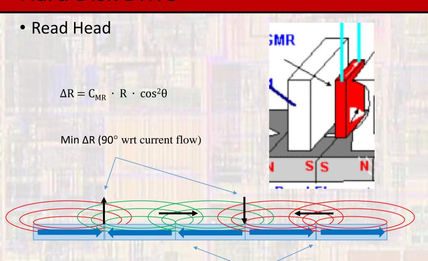
Max ΔR (No component vertical wrt current flow - 0°)
