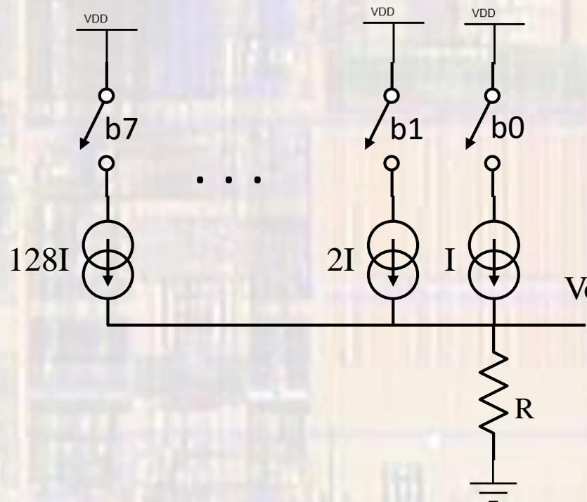
$$V_{out} = (b_0 \times I + b_1 \times 2I + b_2 \times 4I + b_3 \times 8I + b_4 \times 16I + b_5 \times 32I + b_6 \times 64I + b_7 \times 128I) \times R$$
