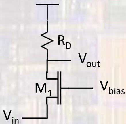
$$I_{D_{M1}} = \frac{1}{2} \mu_n C_{ox} \frac{W_n}{L_n} (V_{Bias} - V_{in} - V_{TH_n})^2$$
