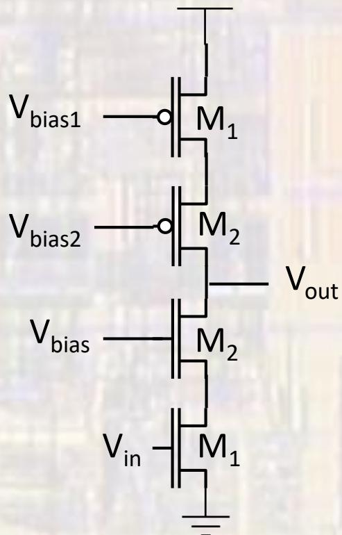
$$A_v = -g_{m1}[(g_{m2}r_{o2}r_{o1}) \parallel (g_{m3}r_{o3}r_{o4})]$$
