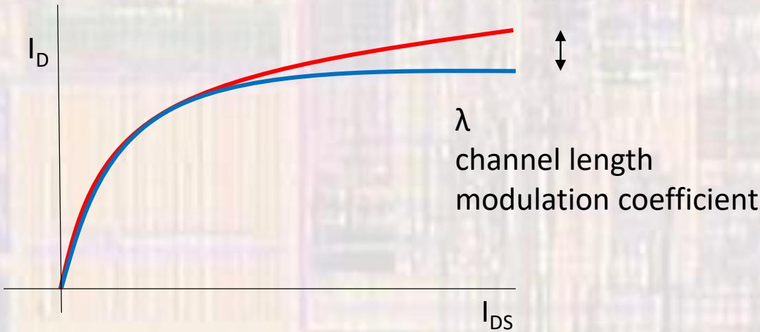
$$I_D = \frac{1}{2} \mu_n C_{ox} \frac{W}{L} (V_{GS} - V_{TH})^2 (1 + \lambda V_{DS})$$
