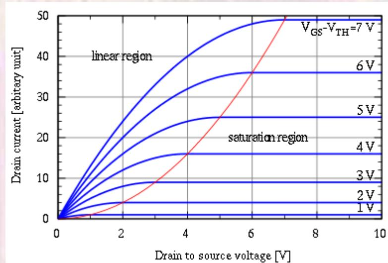
$$I_D = \frac{1}{2} \mu_n C_{ox} \frac{W}{L} (V_{GS} - V_{TH})^2$$
