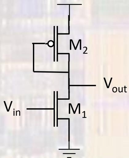
$$A_v = -\sqrt{\frac{\mu_n(W/L)_1}{\mu_p(W/L)_2}} = \frac{|V_{GS_2} - V_{TH_2}|}{V_{GS_1} - V_{TH_1}}$$
