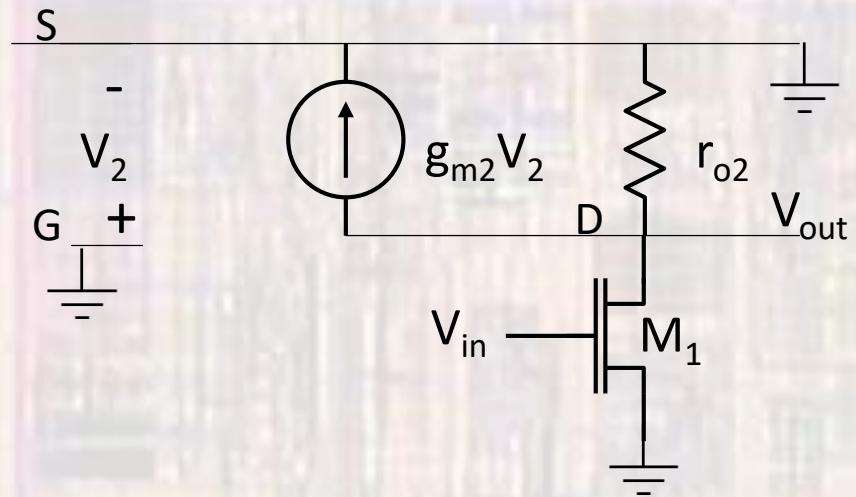
$$A_v = -g_{m1}(r_{o1} \parallel r_{o2})$$
