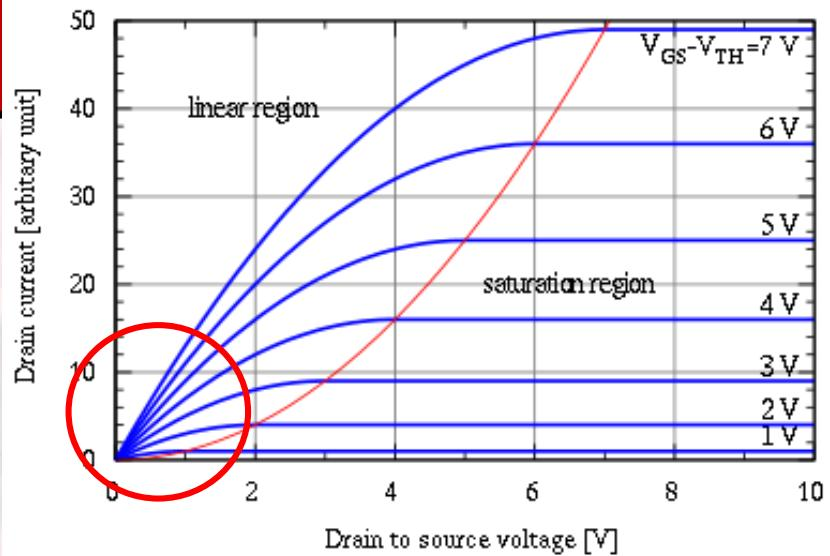
$$I_D = \mu_n C_{ox} \frac{W}{L} \left[ (V_{GS} - V_{TH}) V_{DS} \right]$$
