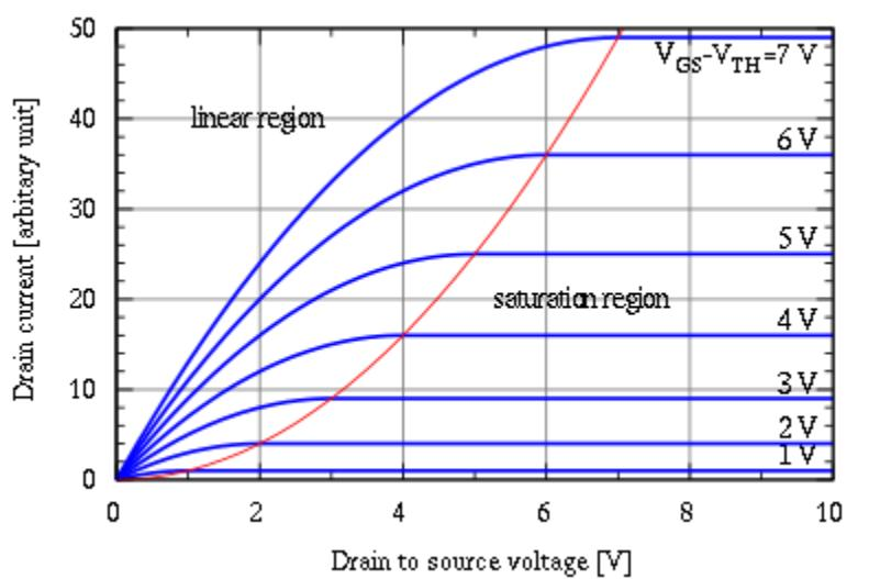
$$I_D = \mu_n C_{ox} \frac{W}{L} \left[ (V_{GS} - V_{TH}) V_{DS} - \frac{V_{DS}^2}{2} \right]$$
