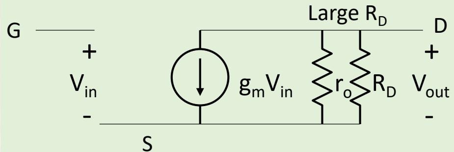
$$A_v = \frac{\partial V_{out}}{\partial V_{in}}$$
