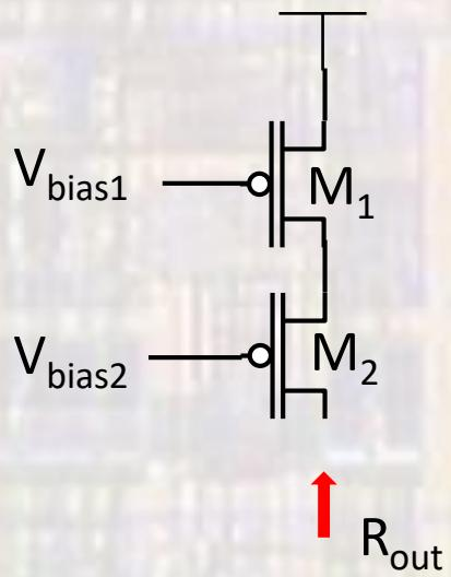
$$R_{out} = [1 + (g_{m2} + g_{mb2})r_{o2}]r_{o1} + r_{o2}$$
