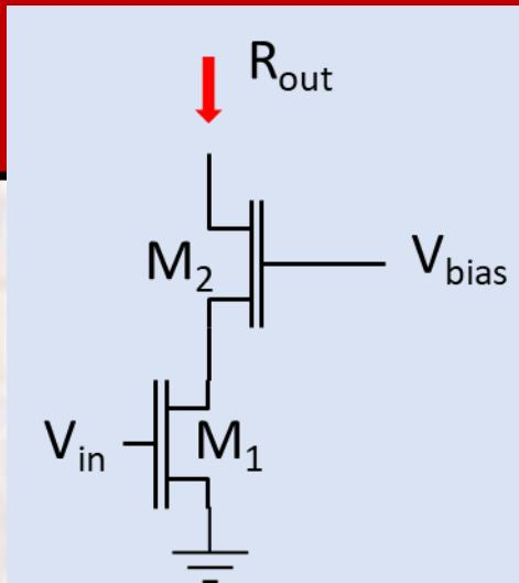
$$R_{out} = [1 + (g_{m2} + g_{mb2})r_{o2}]r_{o1} + r_{o2}$$
