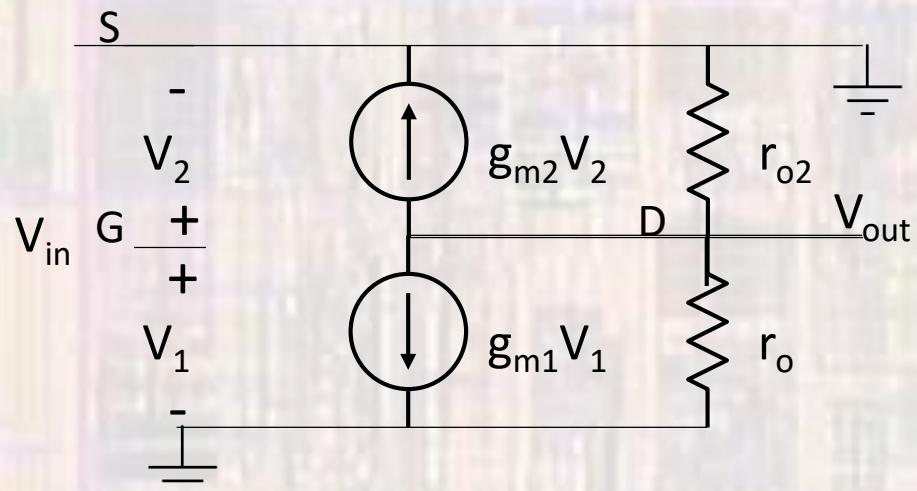
$$A_v = -(g_{m1} + g_{m2})(r_{o1} \parallel r_{o2})$$
