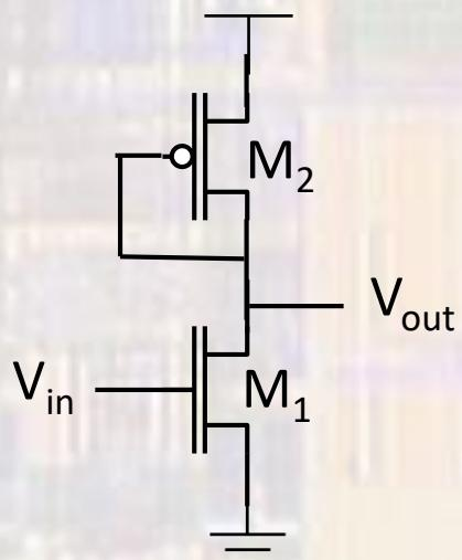
$$I_{D_{M1}} = \frac{1}{2} \mu_n C_{ox} \frac{W_n}{L_n} (V_{in} - V_{TH_n})^2 =$$
