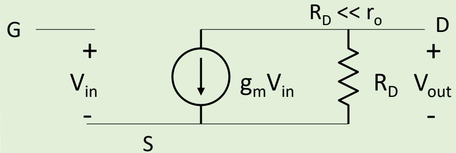
$$A_v = \frac{\partial V_{out}}{\partial V_{in}}$$
