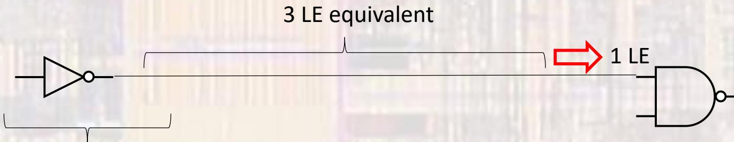
$$t_{pd} = t_{pd_{inv}} + (r \times (3 \text{ LE} + 1 \text{ LE}))$$
