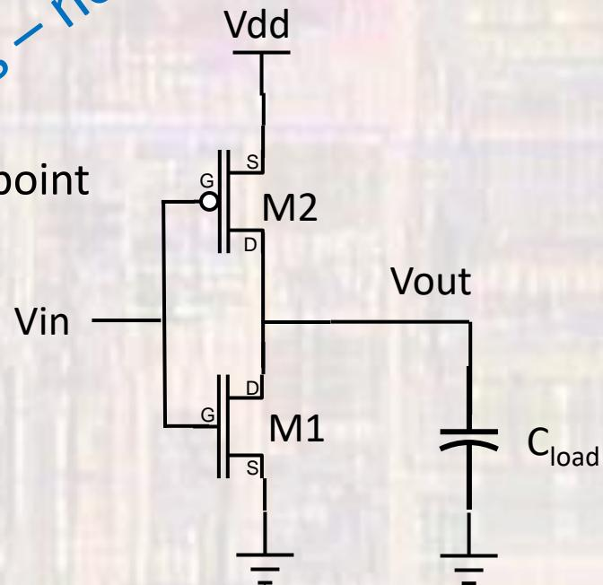
$$t_{lh} = C \frac{1}{\frac{k'_p W}{2 L} (V_{dd} - V_t)^2} \frac{V_{dd}}{2}$$
