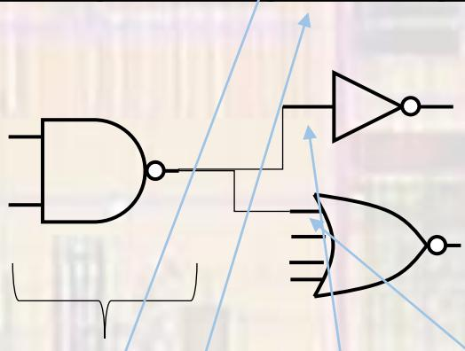
$$t_{pd} = 65\text{ps} + 8\text{ps/LE} * (0.8\text{LE} + 3.33\text{LE}) = 98\text{ps}^{**}$$
