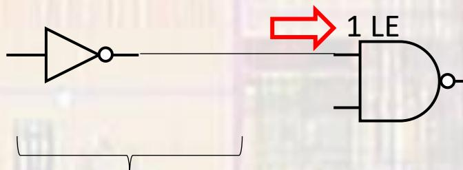
$$t_{pd} = t_{pd_{inv}} + r \times 1 \text{ LE}$$
