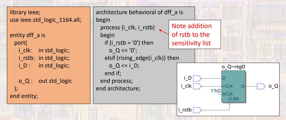
Most of our designs will use DFFs with an asynchronous reset BAR Data Path designs will use DFFs with no reset
