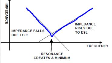
FIGURE 8. IMPEDANCE OF AN ACTUAL CAPACITOR (NON-IDEAL)
