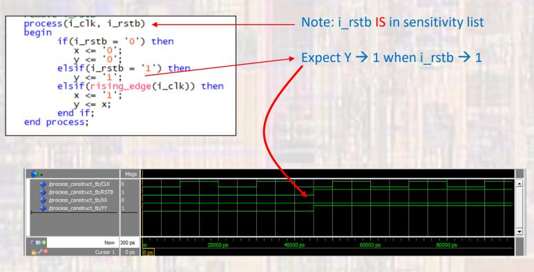
The code is only executed when a signal in its sensitivity list has changed – incorrect version
