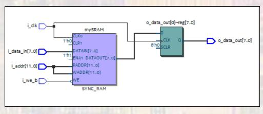
The implementation used inferred SRAM on the FPGA
