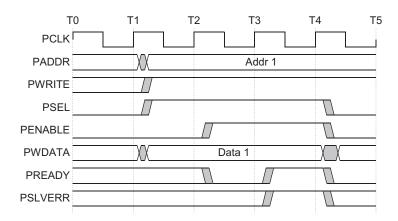
Figure 3-6 Example failing write transfer
