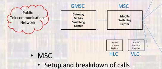
BS **Base Station BSC** Base Station Controller Handles calls between connected mobiles
