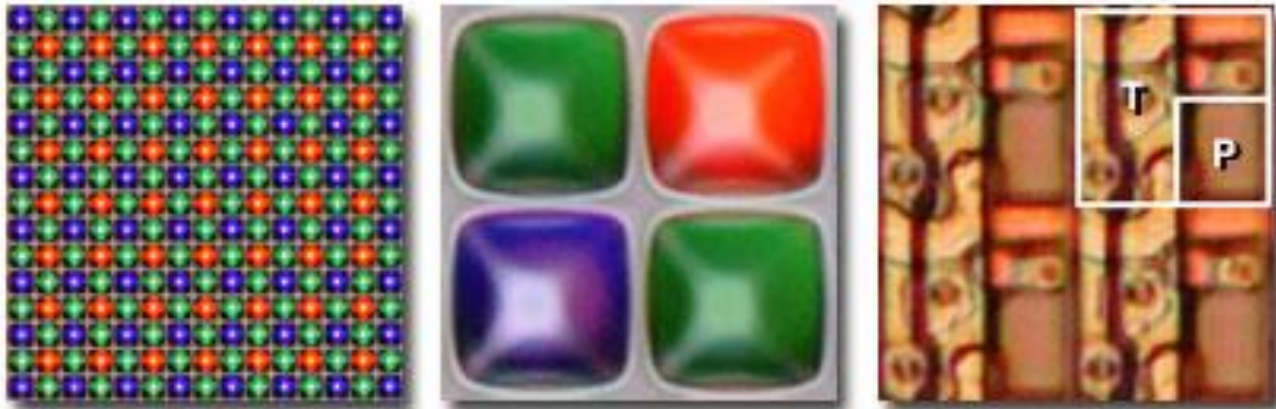
Bayer Color Filter Mosaic Array and Underlying Photodiodes
