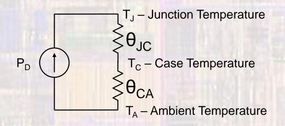
A regulator has:  $\theta_{JA} = 240^{\circ}$ C/W ( $\theta_{JC} = 60^{\circ}$ C/W,  $\theta_{CA} = 180^{\circ}$ C/W) and  $T_{JMax} = 150^{\circ}$ C A heat sink is attached with a new  $\theta_{CA} = 15^{\circ}$ C/W
