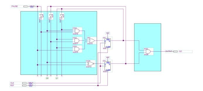
Simulation of the circuit is a little more complex. It would be good to see the state voltages in order to verify the "hold" behavior. Thus, I've added two additional machine outputs and tapped the state voltages.
