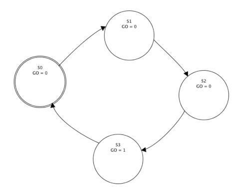
Also **remember** that the data inputs are functions of Q and I: D(Q,I). In this machine there no other inputs.
