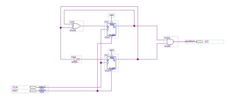
The Moore Machine Model is nicely implemented. The next state combinational logic is in place on the left hand side of the diagram. The state memory is in the middle. The output combinational logic is on the right hand side of the diagram. The common clock and reset signals are attached. Here is the circuit again with the combinational logic blocks highlighted to make them more visible.
