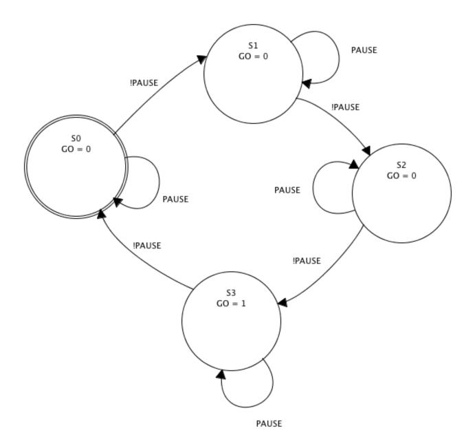
The state diagram shows the new control input on each arrow. The control input determines which arrow gets followed. Each state must have  $2^n$  arrows leaving it where n is the number of inputs. Our previous circuit had no control input and thus  $2^0 = 1$  arrow leaving each state (representing the clock edge transition). Now, the circuit has one control arrow and  $2^1 = 2$  arrows must leave each state: one clock transition arrow for each possible input combination.
