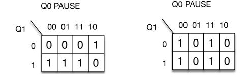
$D1 = \overline{Q1} \bullet Q0 \bullet \overline{PAUSE} + Q1 \bullet \overline{Q0} + Q1 \bullet PAUSE$  $D0 = \overline{Q0} \bullet \overline{PAUSE} + Q0 \bullet PAUSE = Q0 \text{ xnor } PAUSE$
