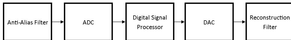
Figure 2: Block diagram of basic DSP system.
